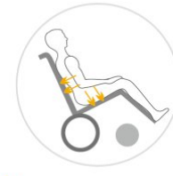
▲ Pressure is distributed when using tilt-in-space
